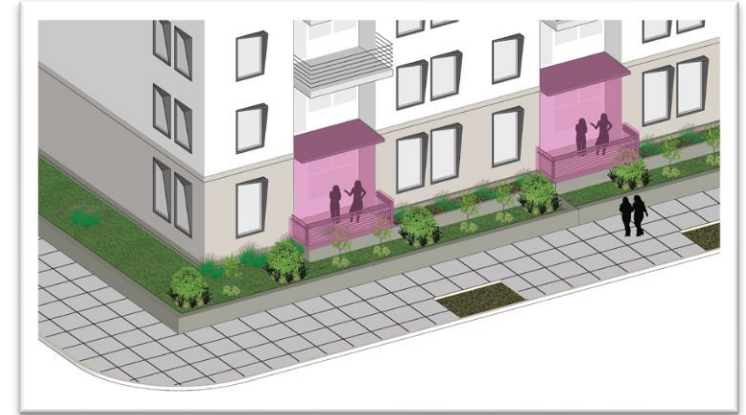
Raised Balcony (no unit entry)
