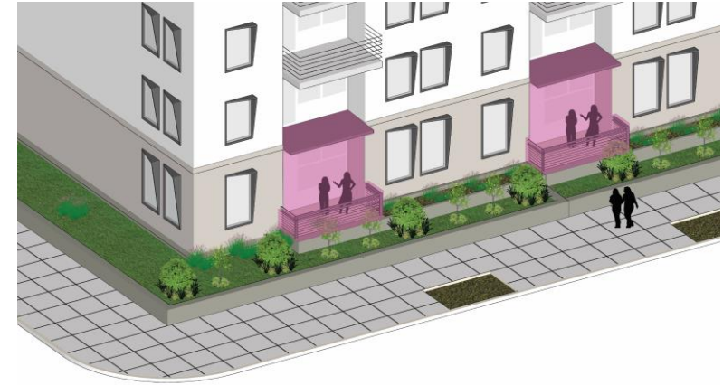
Raised Balcony (no unit entry)
